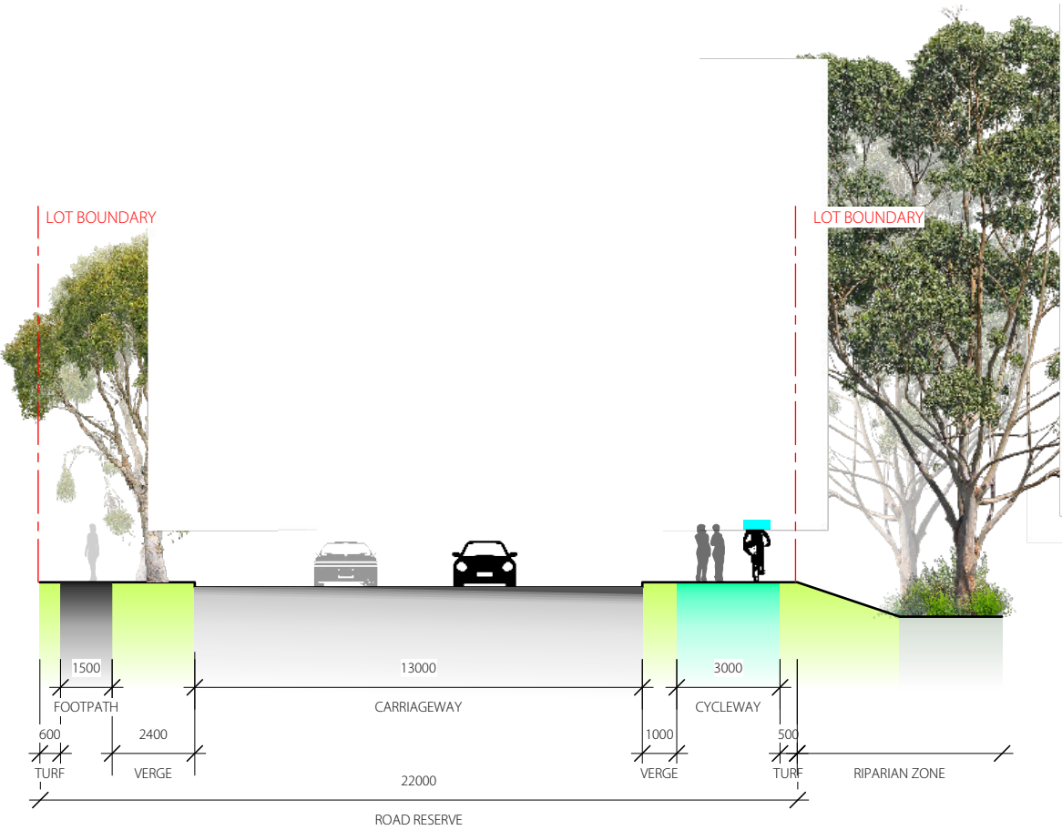
Figure 34. Perimeter Road - Typical Section (Source: Terras)
